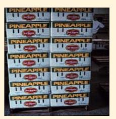
Fig 8. Typical corrugated fiberboard carton used for exporting pineapples.
