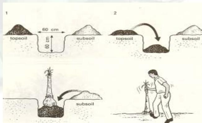
**Fig 5. Preparation of planting holes and planting**
