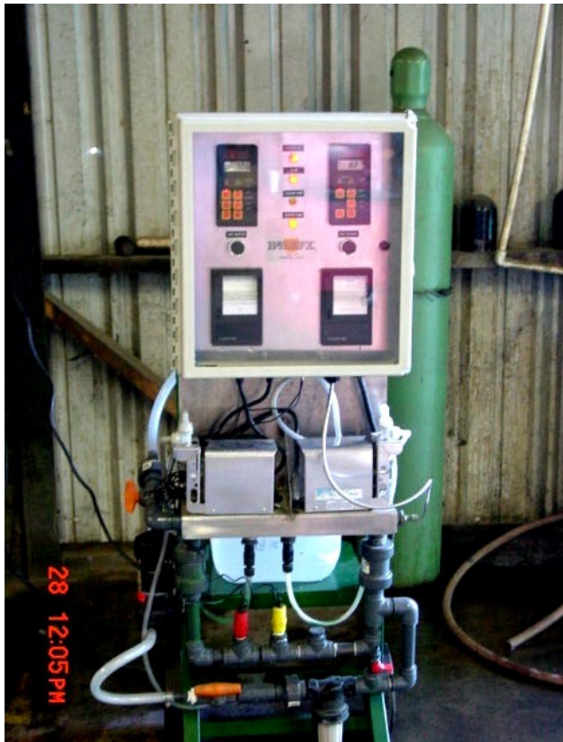
Figure 7. Automated chlorine control and monitoring system that accurately controls and records the chlorine levels in packinghouse wash water.
